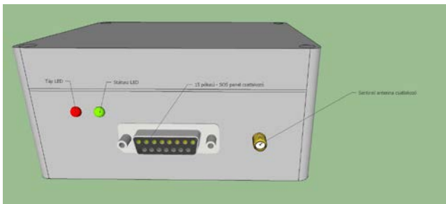
Pic. No. 1.: GPS box Sizes: 115x90x55mm Weight: 340g + pipe clamps 110g
